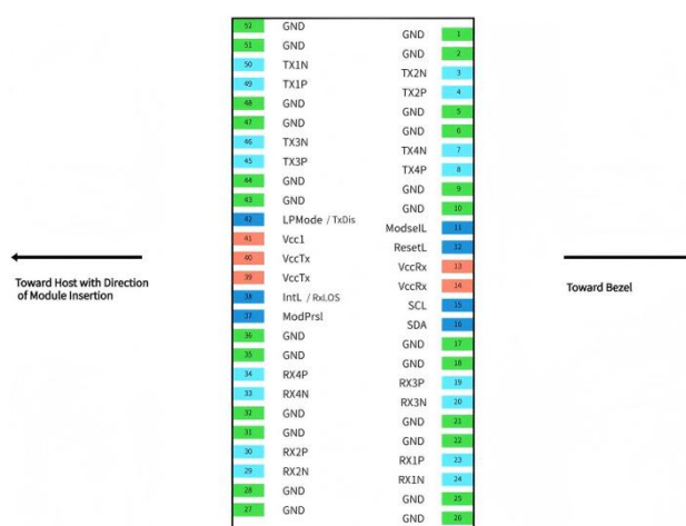
Figure4:QSFP112 Pin view
